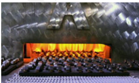
Furnace sintering of the gears produced P/M process
