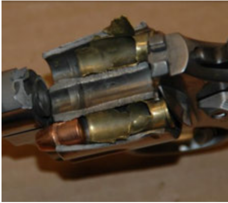
Improper selection of barrel material
