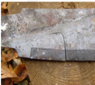
Failed blades due to over loading
