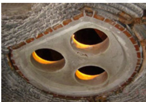
Electric Arc Furnace Refractory lining section.
