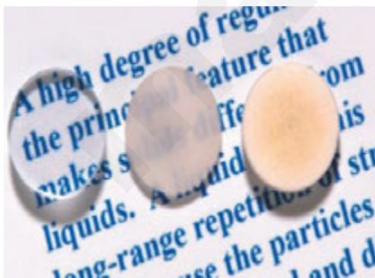
Three thin disk specimens of aluminum oxide, (Specimen preparation, P. A. Lessing; photography by S. Tanner.)
