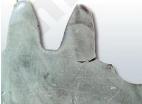
Fatigue failures occur in the tooth root fillet
