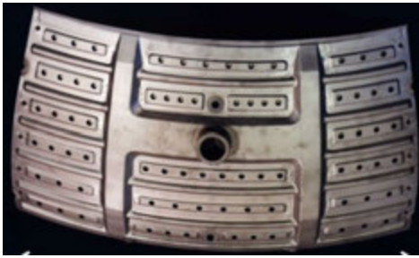
sheet metal engine part made by superplastic forming and diffusion bonding
