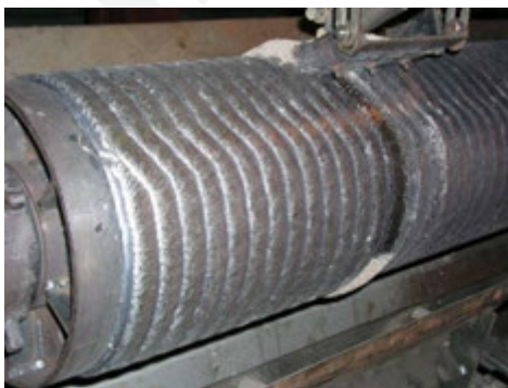
Surface hardfacing for wear prevention
