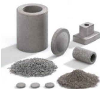
Powders are starting material for PM parts
