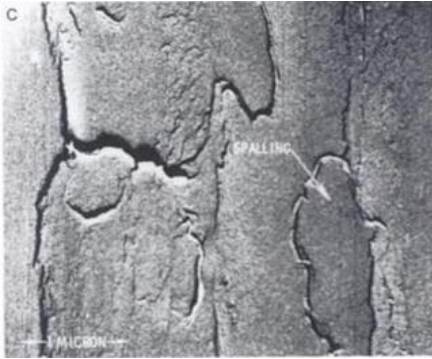
Surface fatigue wear during sliding on metals
