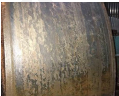
Surface wear of steel rollers due to fretting
