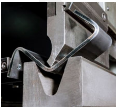
Shaping of sheet metals with mold press
